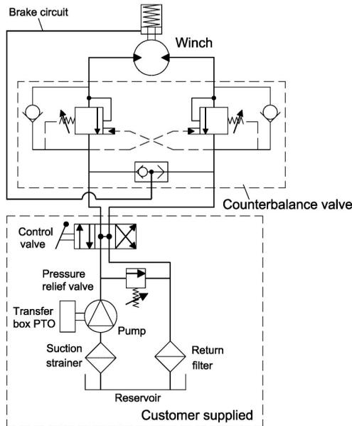
( Powered by PTO / power take off unit driven pump )
